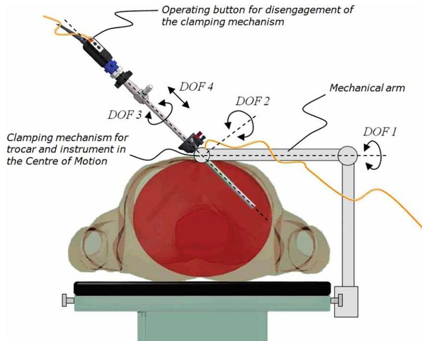
Figure 1. Schematic overview of the novel instrument positioner idea.
