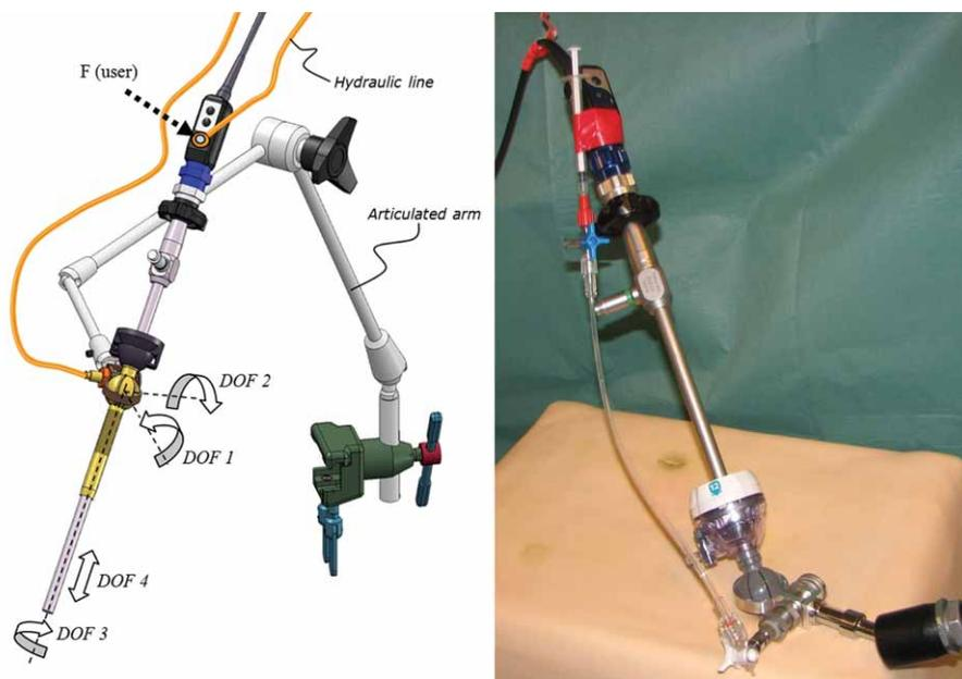
Figure 4. (a) Schematic overview and (b) proof of principle of the deformable ball joint concept.
