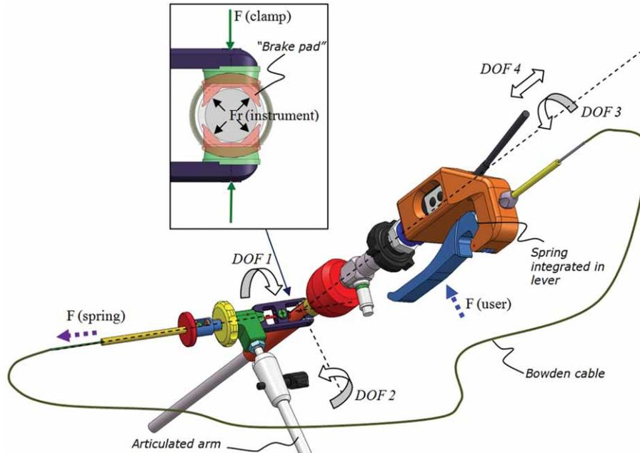
Figure 2. Schematic overview of the scissor mechanism concept and its DOFs.
