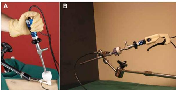
Figure 3. (a) Mock-up and (b) functional concept of the scissor mechanism instrument positioner.
